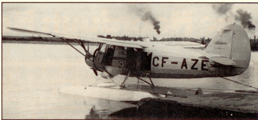
Separate doors for pilot and passengers are shown open on the Mk. II (above); the ladder slides into a slot under the cabin floor. The Mk. VI (below) was produced for the Army as UC-64A and a seaplane version, UC-64B.
