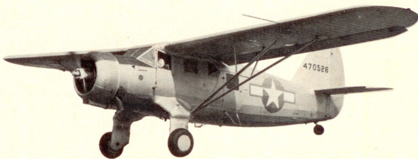
Separate doors for pilot and passengers are shown open on the Mk. II (above); the ladder slides into a slot under the cabin floor. The Mk. VI (below) was produced for the Army as UC-64A and a seaplane version, UC-64B.
