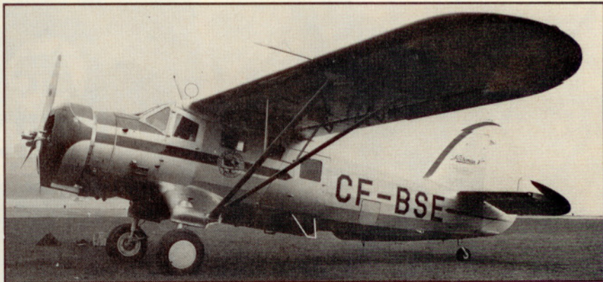
The postwar Norseman was the Mk.V, V standing for victory. It received an extension to the passenger door, a separate baggage compartment door and a three-blade propeller.
