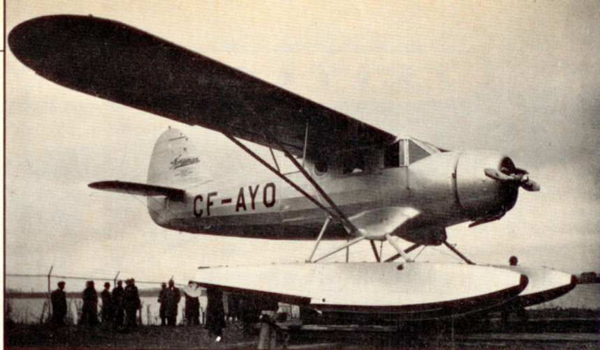
To convince potential customers that the Norseman was designed with seaplane operations in mind, the first flight of the Mark I in November 1935 was made on Edo 6235 floats.
